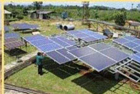
Outdoor weathering tests on PV modules
